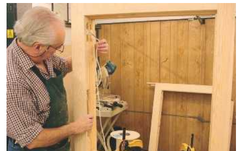
▲ Pic.28 All that remains is to attach the sash cords and counterbalance weights
